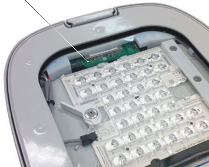
EXCLUSIVE INTERNAL NIC (NETWORK INTERFACE CARD) INSTALLED IN NXT-S LUMINAIRE
